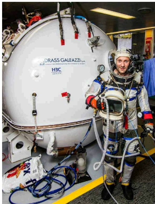
FIGURE 1. (A) Test Subject Standing Before the Trykkammer Wearing the Mark I (Gagarin) Pressure Garment. The orange coverall was not worn in this test; visible is the pressure restraint garment that covers the gas retention layer. Photo courtesy of Jev Olsen, Copenhagen Suborbitals. (B) Test Subject (L) and Pressure Garment Operator (R) During Depressurization Test.
